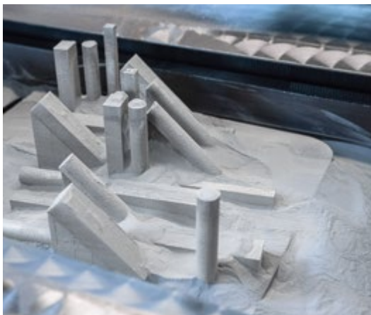
In powder-bed metal additive manufacturing, the workpieces are created layer by layer from powder.
